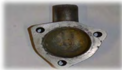
After 5 years with galvanic corrosion wire connection protection fitted.
