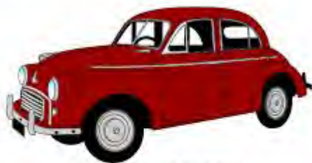
1955 Series II had the new style grille but still retained the split windscreen
