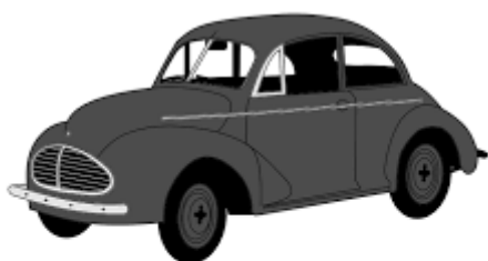
The Mosquito (1943). This prototype which would develop into the Minor had headlights hidden behind the grille
